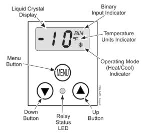
Figure 3: A421 Control Front Panel with LCD and Three-Button User Interface
