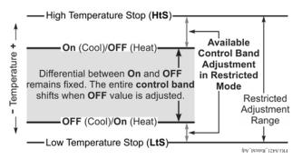
Figure 7: Adjustment Behavior in Restricted Adjustment Mode
