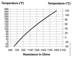
Figure 10: Temperature versus Sensor Resistance
