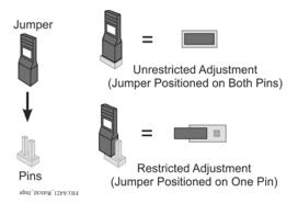
Figure 8: Repositioning the Jumper to Restrict Control Adjustment
