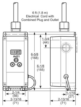
Figure 2: A421 Control with Type 4X (NEMA), IP66 Enclosure Dimensions, in. (mm)
