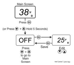
Figure 9: Adjusting Temperature in the Restricted Menu
