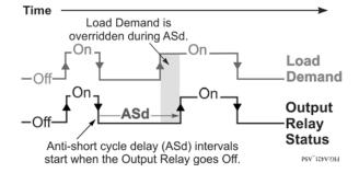
Figure 4: Anti-Short Cycle Delay
