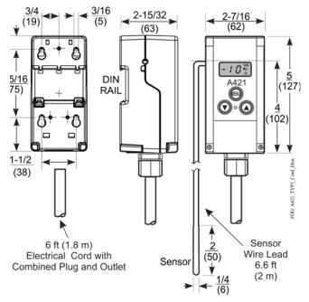
Figure 1: A421 Control with Type 1 (NEMA), IP20 Enclosure Dimensions, in. (mm)
